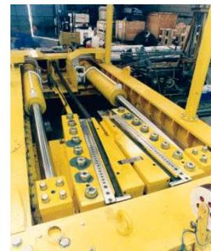
The grippers are specially designed and calculated to give a maximum safety and efficiency and a minimum wire rope wear.
