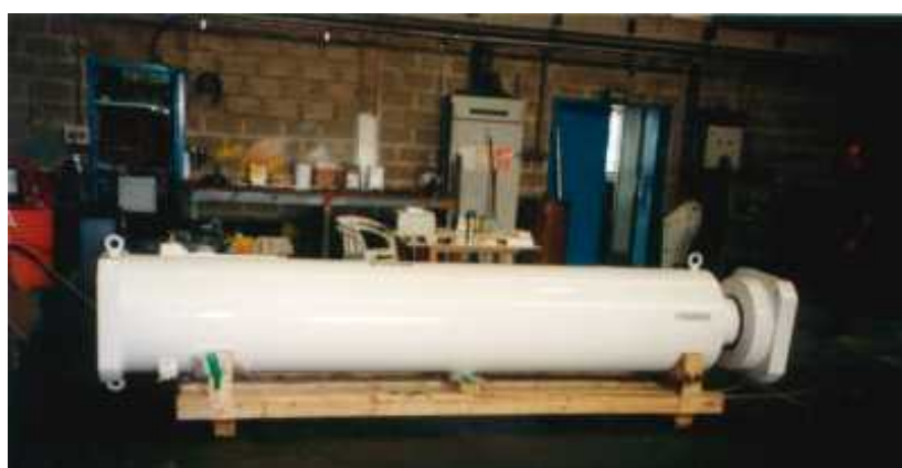
Underwater hydraulic jack - 620 T. 2.5 m stroke.
