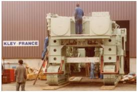
Submarine vehicle for pipeline anchorages
