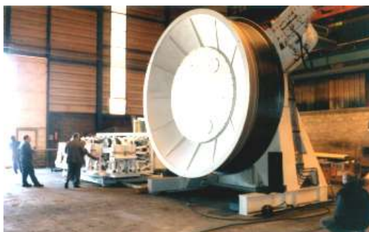
25T - 3.5 m/s Cable Laying Capstan on the "FRESNEL"
