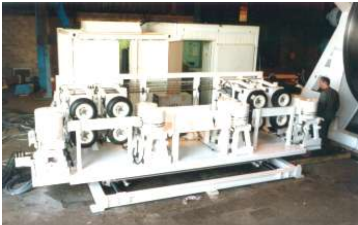
2 T - 3.5 m/s Cable Laying DO/HB on the "FRESNEL"
