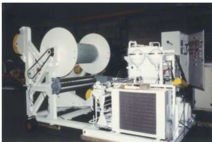
4 T. capstan and 8000 m drum, for handling a 12 mm diameter cable at 2 m/s
