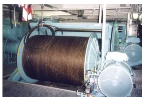
8000 m storage drum with AC electrical motors and frequency converters.
