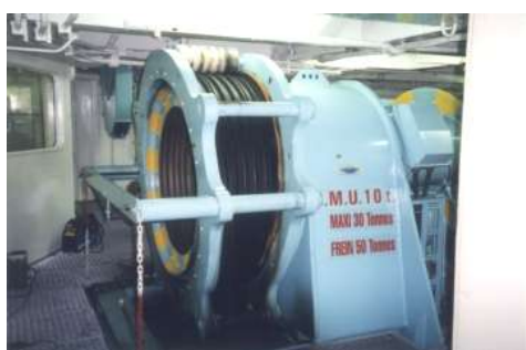
BAND CAPSTAN 30 T. 2.2 m/s - 1.5 m dia.
