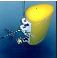
interface, the user can easily and flexibly define the trajectory and sampling schedules. Deployments up to a year or more are possible. Profile patterns can include the full depth of the water column down to 6,000 meters. Mission duration, as calculated from field data and demonstrated in a summer 2001 deployment, is 1 to 1.2 million meters.
