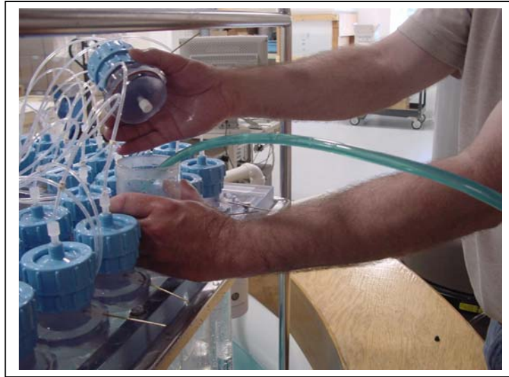
Figure 5-13: Filling the Tubes with Water
