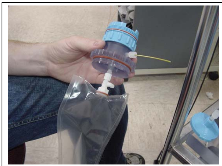
Figure 5-9: Attaching Sample Bag to Sample Tube Cap
