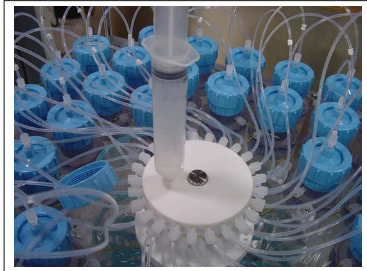
Figure 5-4: Water-Filled Syringe on Valve Intake
