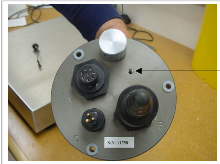
Figure B-2: External Temperature Sensor Installed in Controller Housing
