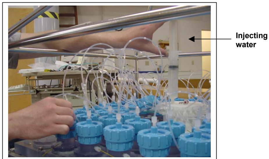
Figure 5-10: Injecting Water into Tubing and Filter Holder
