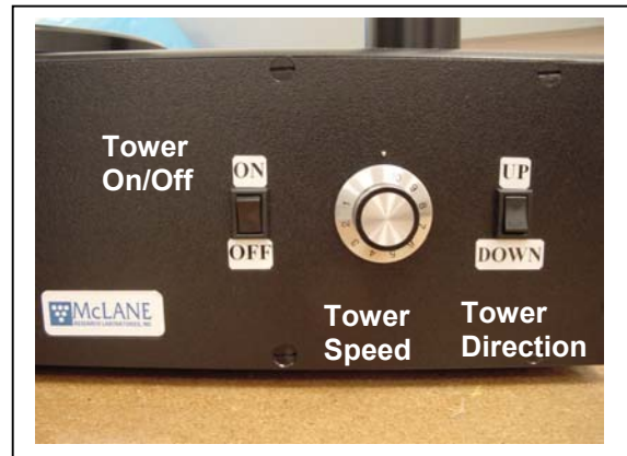
Figure D-3: WSD-10 Tower Controls
