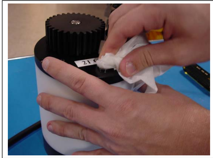
Figure 4-7: Cleaning Excess Oil from Fill Plug
