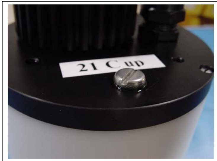
Figure 4-6: Oil Around Fill Hole Screw
