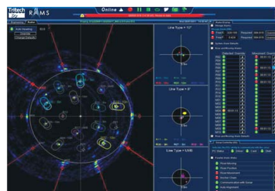
Image showing RAMS™ software screen; here a simulation shows potential alarms in Riser Movement, Anchor Chain, Storage Low and Noise.
